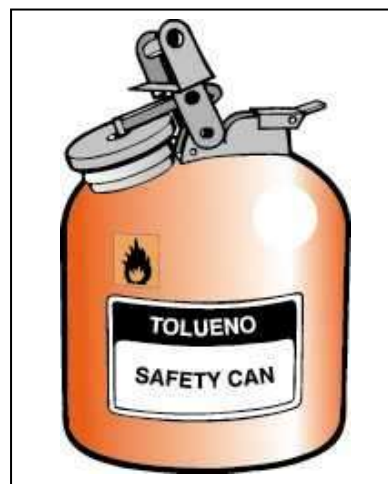
Figure II.23 Safety container for flammable liquids
